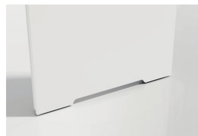
VENTILATION UNDERCUT IN PANEL DOORS* undercut 15 mm - for rooms with recuperation undercut 26 mm - WC for doors 80'-100' undercut 38 mm - WC for doors 60'-70'
